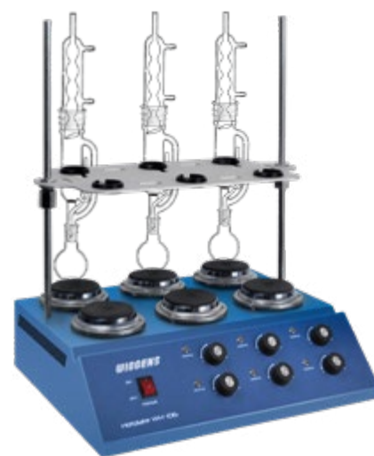
Parallel reaction for Soxhlet extraction
