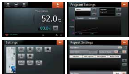
4" Full Touch Screen TFT LCD (Smart-Lab™ Controller)
