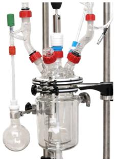
The Lab Fast Pro Reactor was designed by collective efforts of chemists and engineers for chemists. It allows to work with vessels of different sizes by changing the glassware in mere minutes, not hours. A unique frame design and vessel geometry allow to replace only the vessels themselves, keeping all the other glassware and accessories in place.
